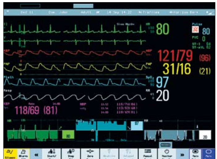
Horizon trends are the distinctive shaded trends running along the bottom of the screen. Note how the colors are keyed to the live waveforms.
